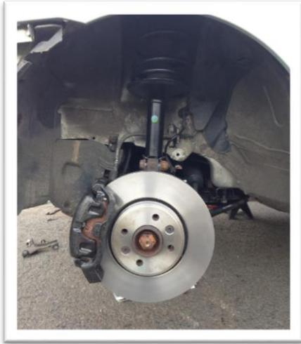
Bolt the above onto the car making sure the rad mountings are lined up. I won't go through some of the reassembly but do back up what you've undone/taken off!
