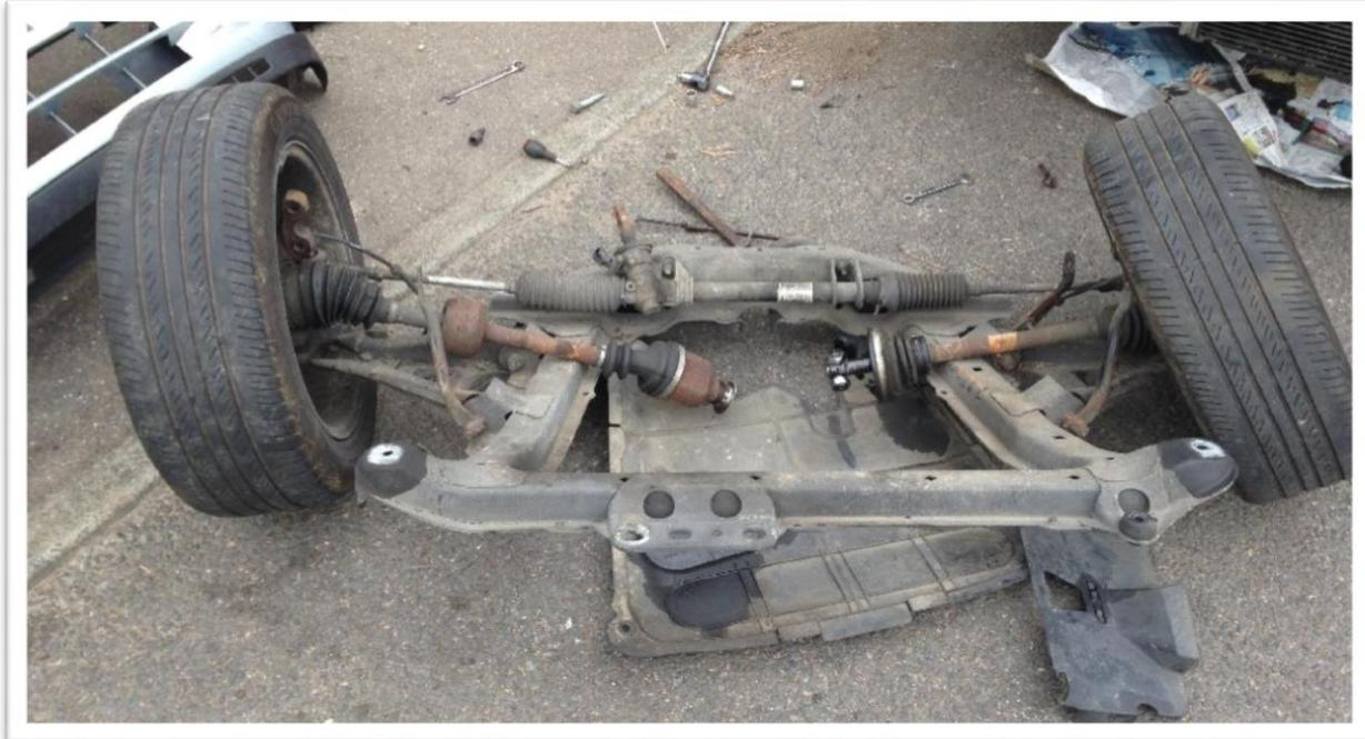
Take the old steering rack off and put it onto your new subframe set up. It's a vesy good idea to make sure the track rod ends are nice and loose for adjusting when on the car. Get a wire brush on them and copper slip the threads.
