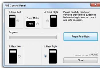
While the solenoid valve is operational, gently depress the brake pedal (without it reaching its travel limit) and release slowly.
