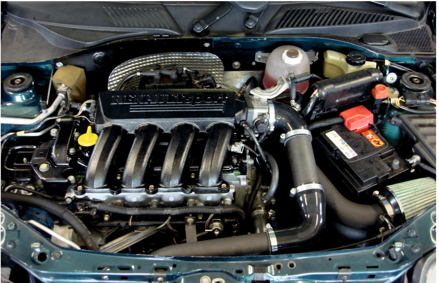
A few pictures of the intercooler and pipework. This clearly shows the intercoolers location and pipe run. The intercooler mounts through the cross member, so you need to drill through both upper and lower metal skins.
