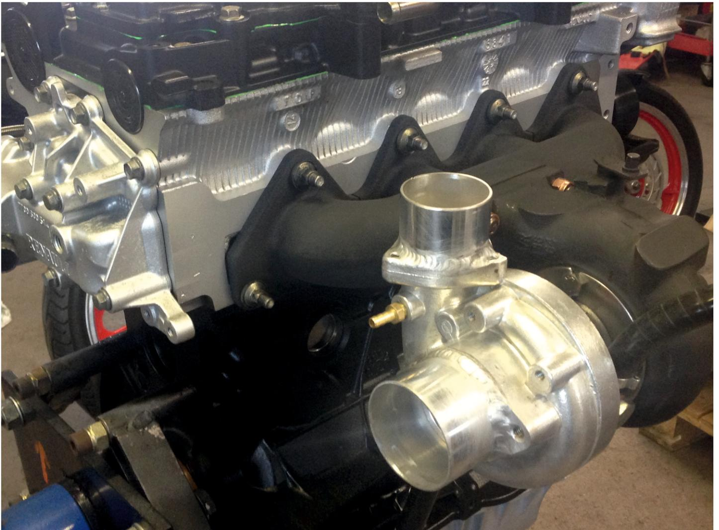
Connect drain hose between block and turbo.
