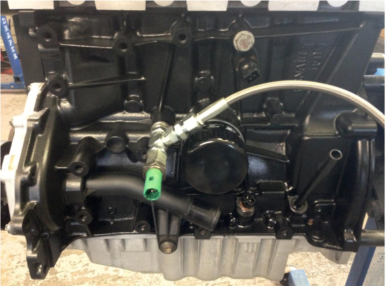
Check all fittings and then connect to the turbo, it's a good idea to pre oil the turbo before finally connecting the feedpipe. Once this is done refit the actuator and start on the intercooler / pipework.
