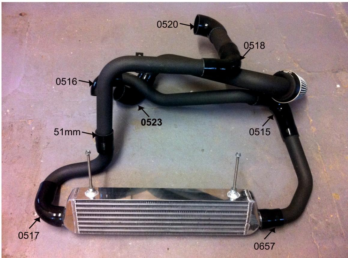
**Phase 1 Models: Completely remove the breather pipe that runs to under the throttle body and fix Blue Blanking bung under throttle. Install our breather pipe from the outlet on the back of the engine and route to front of vehicle.**
