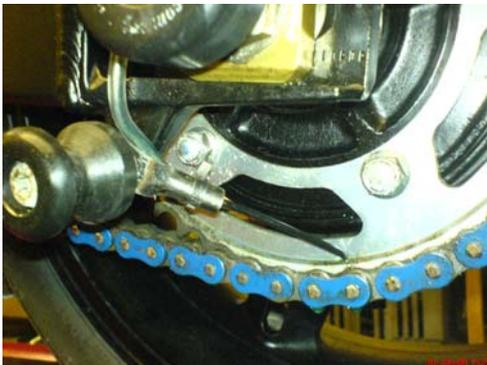
The Dispenser Assembly, shown left, is routed along the Swingarm using Dispenser Mounting Sleeves & Glue and secured to the paddock stand bobbin mount using a cut down Dispenser Plate, part numbers 19 & 20.
